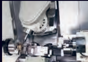
Mill/Turn by B-axis tool spindle
